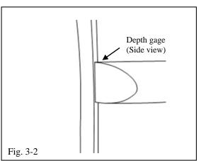
Align the adjustment tool to the edge of the door, with the angle edge positioned toward the inside of the door (Fig. 3-2).
