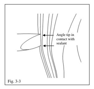
Align the adjustment tool to the edge of the door, with the angle edge positioned toward the inside of the door (Fig. 3-3).
