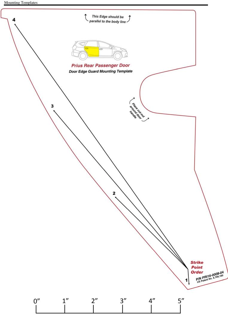
Dealer Installation Note: Check the above scale to ensure it is 1:1. Adjust on photocopier if it is not to scale. If this is a pdf document, set the "Page Scaling" to "None" in the Print dialogue box prior to printing.
